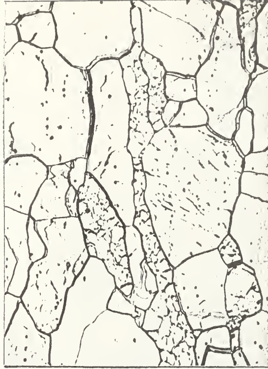
FIG. 28 AT 540°C, UNDER .6%/HR. STRAIN RATE, FOR 30 HOURS (ROCKWELL 30T 40.7)
